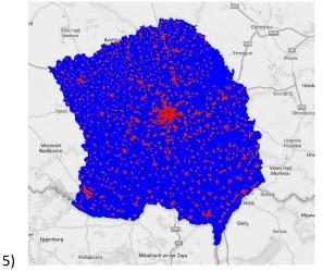
6) Resulting grid has a lot of blue cells that correspond to zero population value. It is possible to ignore zero input values during gridding process. This can be done by clicking on Data Conditioning Options button (next to Select Columns dropdown). Select Specify Invalid Data option, click on Insert Row and leave zero as an invalid data value. Click Ok and click Process to repeat gridding operation.
