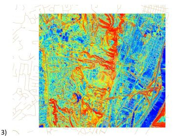
A) Next step is to find all areas that have a slope higher than 4 degree. We will use Classify tool to create classify grid with only one class "High Slope" that would include all areas with a slope 4 degrees or high. You can use the same values for classification as shown below:
