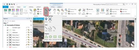
Or you can use the *Insert* dropdown on the *SPATIAL* tab where it also contains the Insert/Create tools from *MapCAD*.
