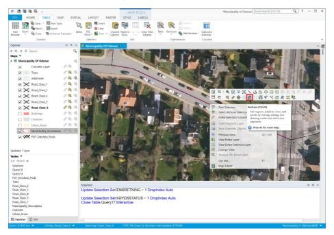
Now you can see the individual nodes of the selected object and using the *Select* tool you can select these nodes and move them using the mouse or delete them using the *Delete* key on your keyboard.
