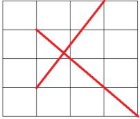
But the intersection between the two red lines isn't located at an intersection of the black lines. If you were to create a node at the red intersection, it will be moved to the nearest black intersection.
