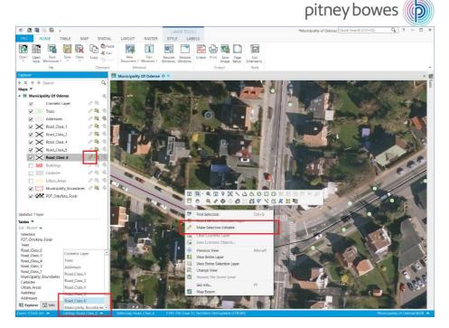
It is important to notice that you can only have a single layer editable at any time in each map window. You can however have multiple map windows with different editable layers and switch between these map windows.
