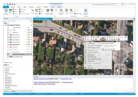
You can enable *Snap* using the S-key on your keyboard to snap an existing or new node to another node in the same layer or in a different selectable layer.
